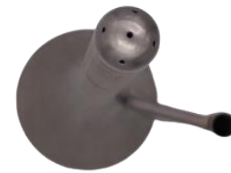
Figure 1 Air Data Boom Head
